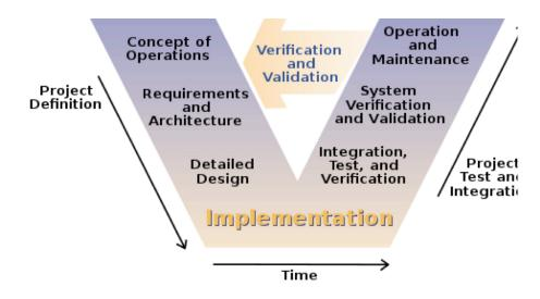
Figure 2: The V-model of system development, often referenced in safety critical standards such as ISO 16508 and 26262.
