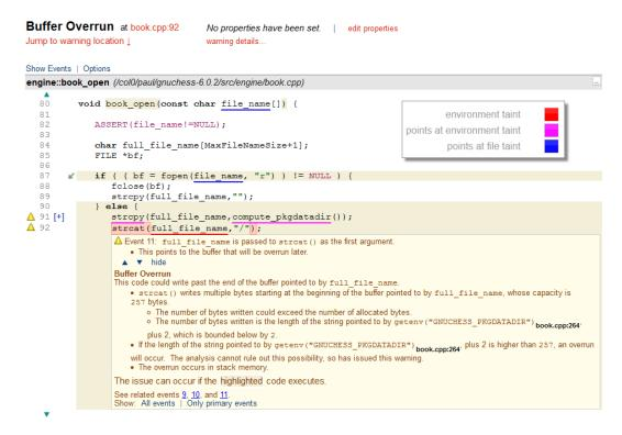
Figure 2. A buffer overrun warning where the underlining shows the effect of taint.
