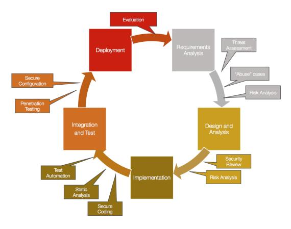
Figure 1: Security processes superimposed over the software design lifecycle.
